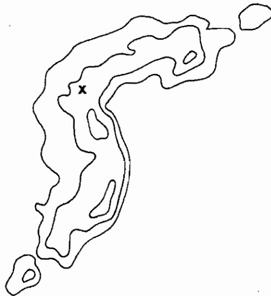
Fig. 4. LEWP (line-echo wave pattern) . Typical radar reflectivity contours associated with a LEWP. The crest of the wave pattern is at X. Note similarity of the echo below X to the bow echo in Fig. 1.
